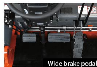
Wide brake pedal Optimized pedal layout improves operation comfort (hydrodynamic truck).
