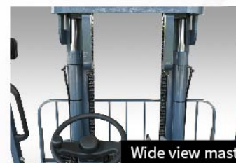
Wide view mast Optimized mast structure effectively improves driver's view.
