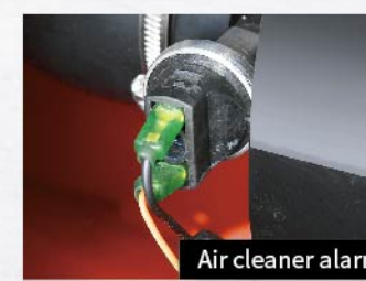
Air cleaner alarm Standard configuration of air cleaner alarm reminds customer to maintain the air cleaner in time so as to protect engine and improve engine reliability.
