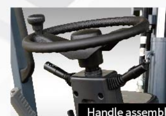
Handle assembly Standard configuration of combined handle integrating electro hydraulic reversing handle, steering and lights facilitates operation (hydrodynamic truck).
