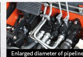
Enlarged diameter of pipelines Enlarged diameter of hydraulic system pipelines reduces pressure loss and prolongs hydraulic system service life.
