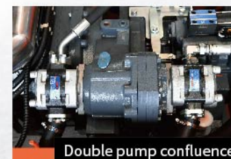
Double pump confluence The application of double pump confluence hydraulic system provides oil supply as required and reduces energy consumption of the whole truck.
