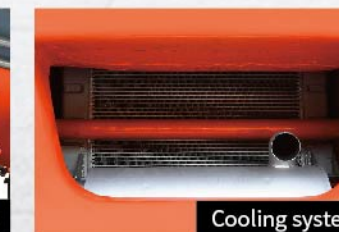
Cooling system Enlarged aluminum plate fin radiator makes three kinds of temperature are controlled in a good range and effectively improves the reliability of the system.
