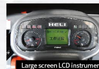
Large screen LCD instrument Large screen LCD instrument overally monitor truck state. The instrument displays real time engine and truck fault information and humanized reminder.
